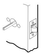
4 Drill and fit 4 wood screws for alignment only
