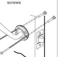
Fit through bolt fixing
