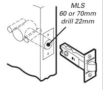
3 Fit spindle through latch
